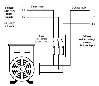
The disconnect switch controls the L1-L2 input supply line to the converter and isolates those lines from the load. All three output lines are de-energized as long as the switch remains off. This control arrangement requires the disconnect switch be sized large enough to withstand the entire 1-phase input current to the load.
