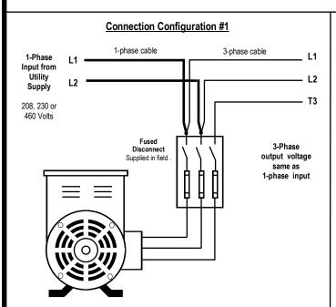
This connection arrangement allows the L1 & L2 line to remain energized regardless of whether the converter is operating. It is used where any downstream load equipment requires continuous single-phase service. The converter must be started and running to operate any 3-phase load.
